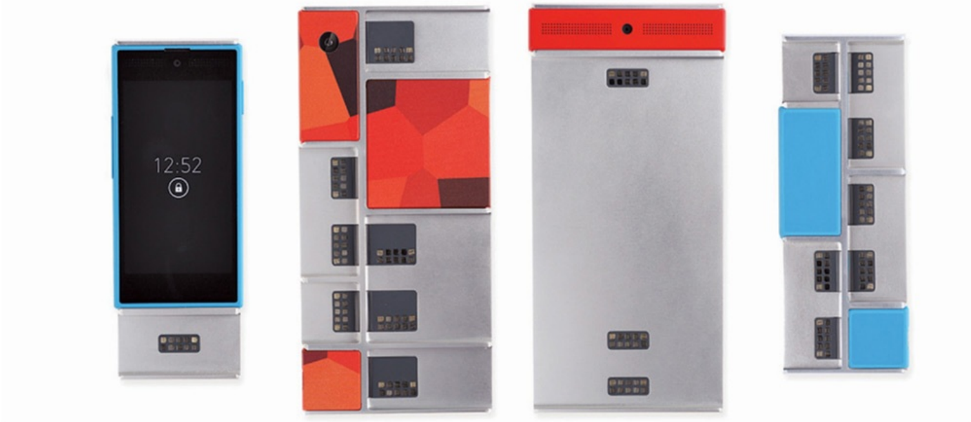
Google's Project Ara is reinventing the cell phone using modularity. This should reduce costs and open innovation.
